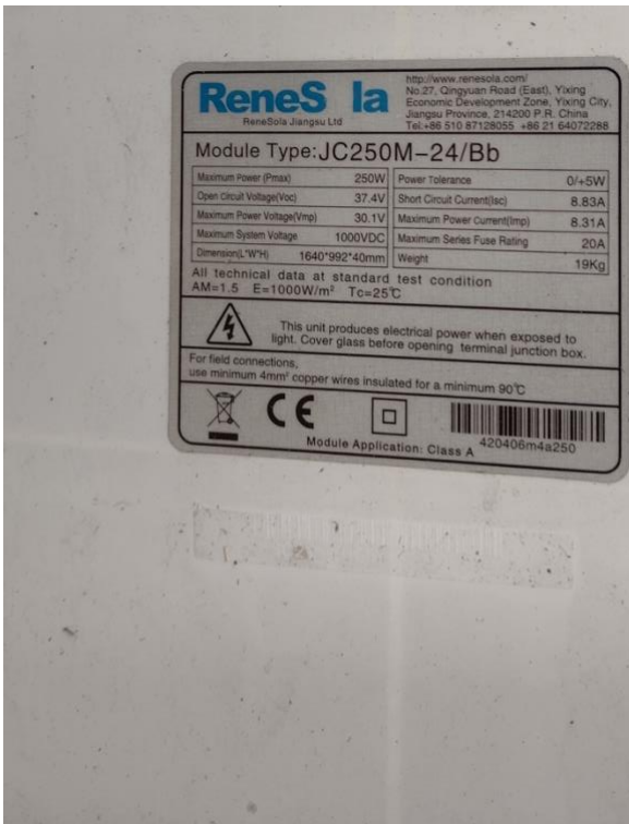
2110-CPV-001-019 *example of serial number sticker on backsheet worn away
