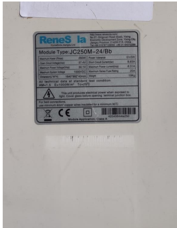
2110-CPV-001-024 *example of serial number sticker on backsheet worn away
