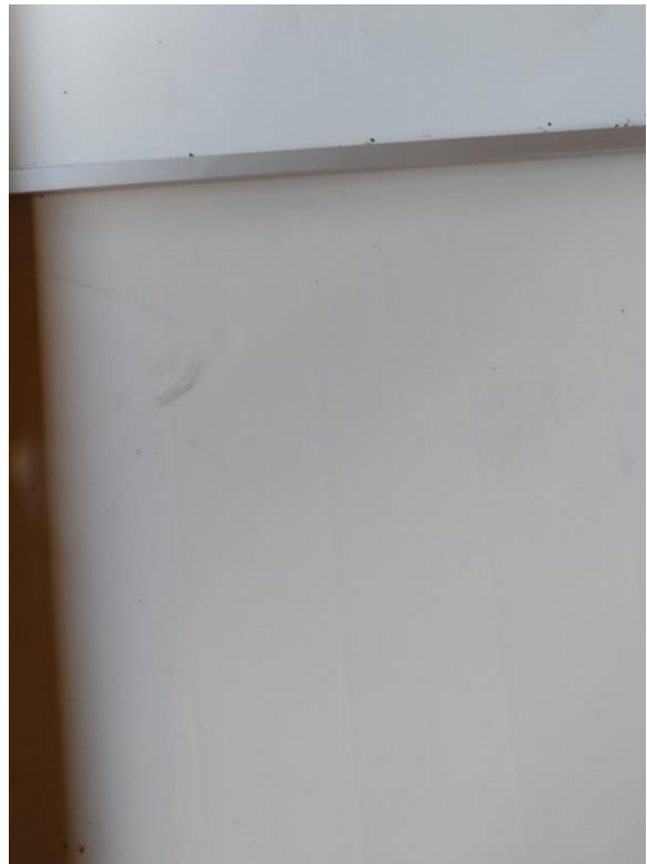
2110-CPV-001-021 * minor dent in backsheet
